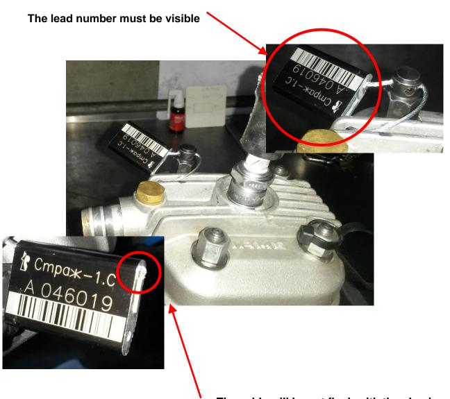
The cable will be cut flush with the aluminum part of the seal
